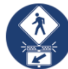
Rectangular Rapid Flashing Beacons (RRFB)
