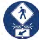
Rectangular Rapid Flashing Beacons (RRFB)
